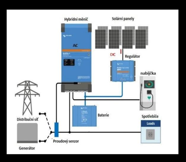
The main component of hybrid power plants is the Hybrid Inverter, which has an input from the batteries for island mode and an input from the distribution network for switching to this backup.
